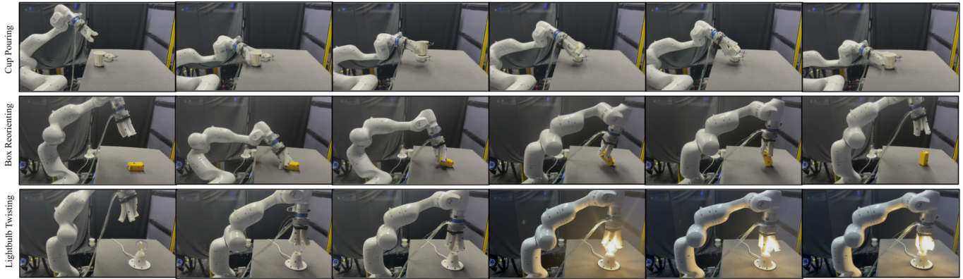
Fig. 7: Real-World Manipulation Results. Sequential frames showing zero-shot real-world execution of contact-rich manipulation tasks with SoftAct , including paper cup pouring, box reorientation, and light bulb screwing. The robot successfully maintains stable contact and executes task-relevant object motion despite severe embodiment mismatch between the human demonstrator and the non-anthropomorphic soft robot hand.
